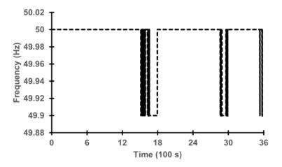
Fig. 8 Frequency profile of the split inverter air conditioning (AC) system under at an 18°C temperature setpoint
