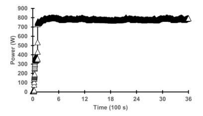
Fig. 6 Power profile of the split inverter air conditioning (AC) system under at an 18°C temperature setpoint
