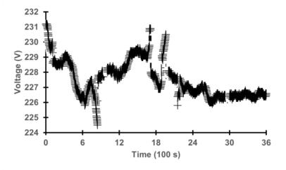
Fig. 4 Voltage profile of the split inverter air conditioning (AC) system under at an 18°C temperature setpoint
