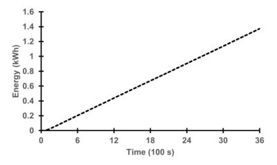
Fig. 7 Energy consumption profile of the split inverter air conditioning (AC) system under at an 18°C temperature setpoint
