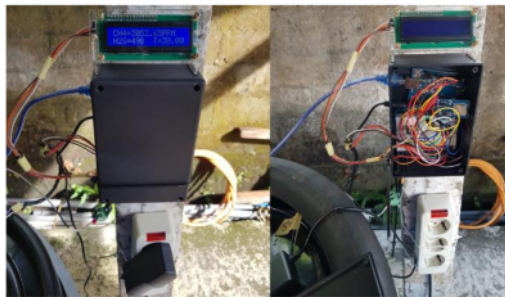
Figure 3. Actual implementation of the microcontroller system with integrated sensors Source: Author's analysis (2023)
