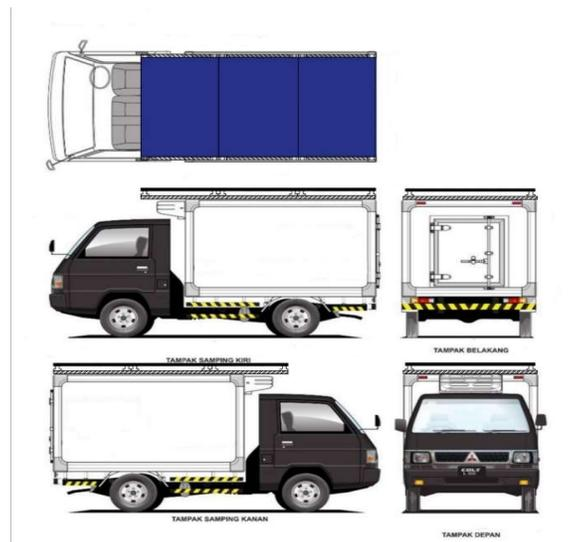
**Gambar 6** Karoseri Box Kontainer Mobil
