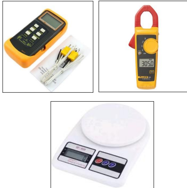
Gambar 2. Instrumen penelitian (thermocouple, tang ampere, dan timbangan digital)
