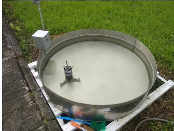
Figure 6. Overall View of the Open Pan evaporimeter Monitoring System Alat
