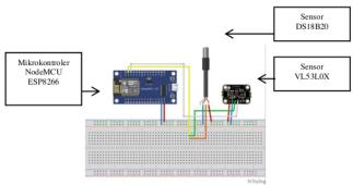
Figure 4. Thingspeak Wiring Diagram with Fritzing
