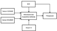
Figure 1. Monitoring System Hardware Block Diagram
