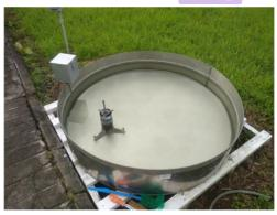
Figure 6. Overall View of the Open Pan evaporimeter Monitoring System Alat
