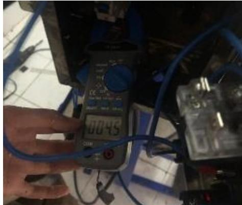
**Gambar 4. 4** Mengukur kuat arus
