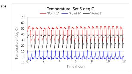
Fig. 8. Average temperature on each point investigated : (a) set at  $0^{\circ}$ C and (b) set at  $5^{\circ}$ C.
