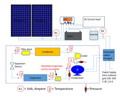
Fig. 3. Schematic diagram of experimental rig and measurement positions.
