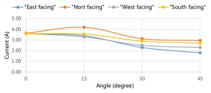
Fig. 4. Variation of current (I) with combination of facing and angles.
