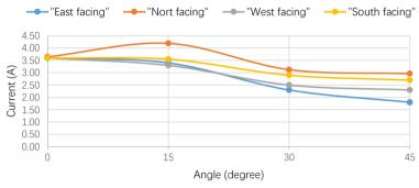
Fig. 4. Variation of current (I) output with combination of facing and angles of photovoltaic array at Bali State Polytechnic-Bali Indonesia
