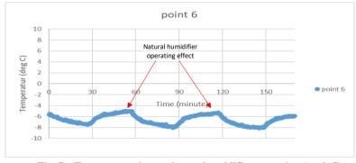
Fig. 7. Temperature increasing on humidifier operating (set  $0^{\circ} C$ )
