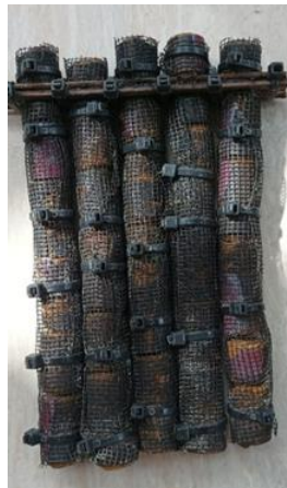
Figure 3. Sintering zeolite cooling pad
