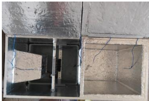
Figure 2. Evaporative cooling system
