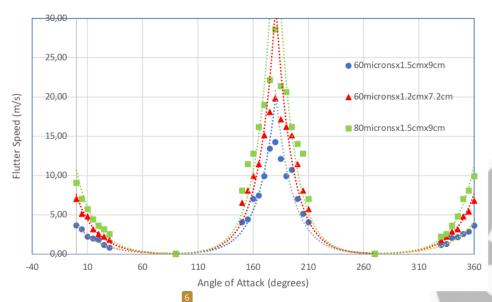
Figure 3. The effect of the angle of attack to the flutter speed
