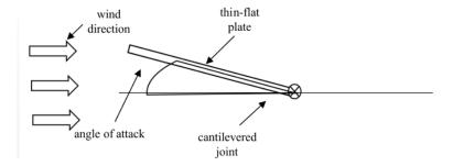
Figure 1. Experimental setup diagram
