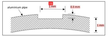
Figure 1. Physical dimension of grooves.
