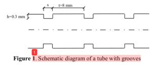
Groove with rectangular surfa and circumferential pattern were arranged on outer sur 2 ce of tube side or in the annulus room of the double pipe heat exchanger. The groove depth (h) was 0.3 mm, the
