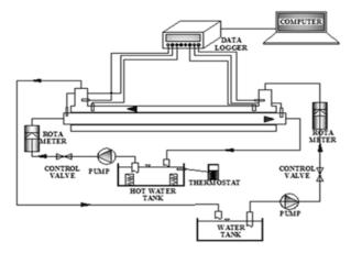
Figure 2. The schematic representation of the apparatus set-up
