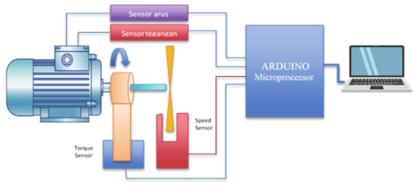
Figure 4: Speed and torque measuring circuit.
