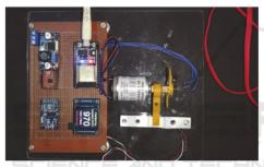
Figure 6: Circuit are made for measuring speed and torque.
