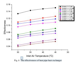
Results of the experiment are to determine the effectiveness HPHE with variations or operating parameters as shown in Fig. 6. It illustrates that the greatest effectiveness 0.15 was obtained when using six rows HPHE with the air velocity 1 m/s at a temperature of  $45^{\circ}$ C. At the same condition showed that the evaporator inlet air temperature has decreased to  $2.4^{\circ}$ C. Moreover, the
