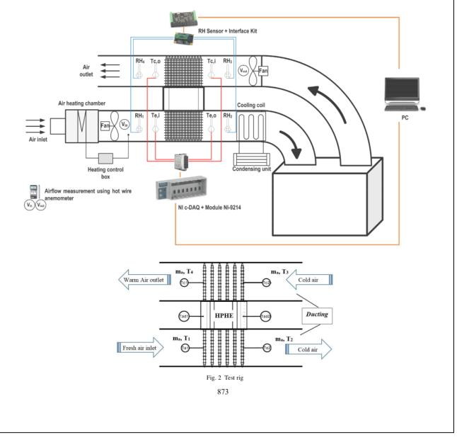
simulator, and several measuring devices that are connected to ducting with dimensions of 300 mm x 470 mm. The placement of heat pipes in the ducting and direction of airflow in and out also shown in Fig. 2.
