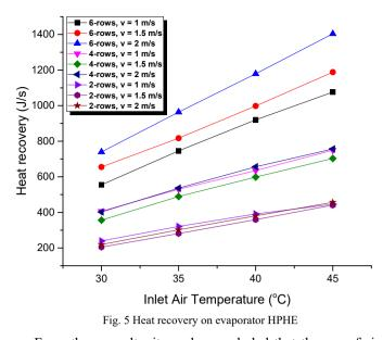
From these results, it can be concluded that the use of six rows HPHE was an optimum design compared to the use of two or four rows. The addition of air velocity will increase the mass flow rate of air that can increase the heat transfer rate between the air and HPHE thus increasing the value of heat recovery.
