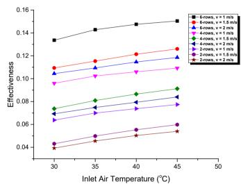
Fig. 4 The effectiveness of heat pipe heat exchanger
