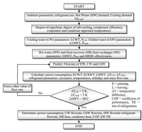
Figure 2. Flowchart of numerical models in EES for the water cooled chiller with hot water heat recovery system
