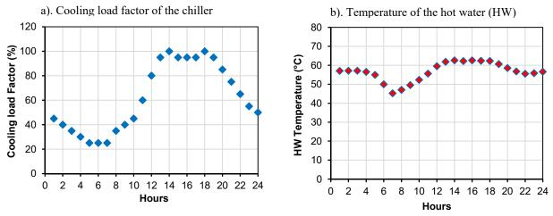
Figure 4. Hourly variation of cooling load factor of the chiller and hot water temperature produced from the heat recovery (HR) system
