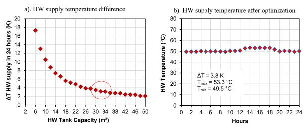
Figure 8. HW temperature difference at various storage tank capacity and variation of HW temperature after optimization
