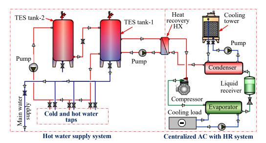
Figure 1. The concept of the hot water supply system with heat recovery central air conditioning system and hot water storage tank
