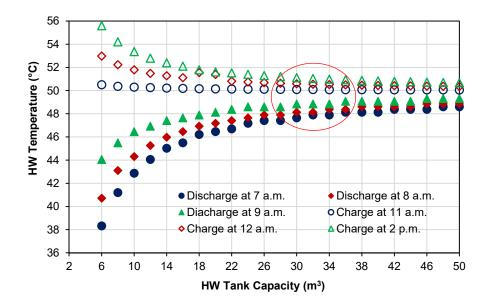
Figure 7. Variation of hot water temperature after charging and discharging processes at different capacity of the storage tank
