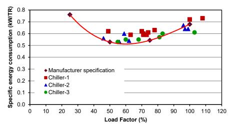
Figure 5. Variation of chiller system energy performance at different load factor
