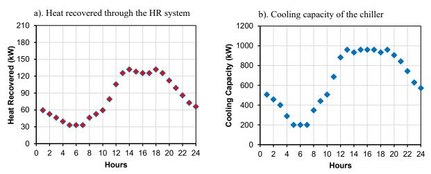
Figure 3. Hourly variation of heat recovered through the HR system and cooling capacity of the chiller
