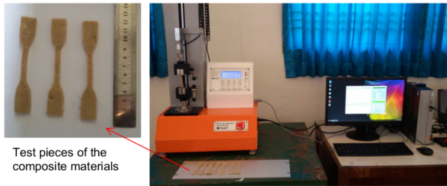
Fig. 3 Tensile testing machine with test pieces
