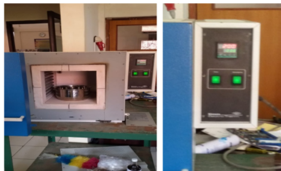
Fig. 2 Electric melting furnace completed with digital temperature controller
