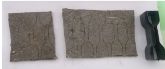
Fig. 1 A sample of test specimen for composite material in fourth composition category
