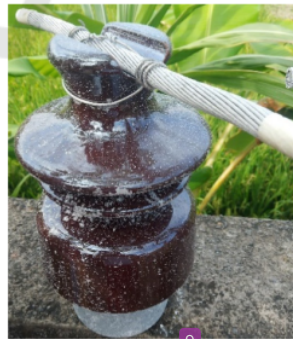
Figure 3: Dry dummy pollution on the surface of pedestal insulator.
