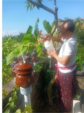
Figure 2: Dummy pollution spraying process.
