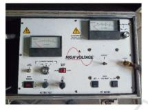
Figure 5: High voltage VLF hi-pot instruments.
