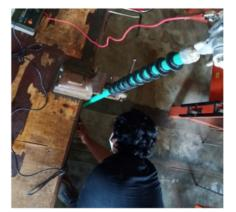
Figure 4: Wet insulation resistance pretest with megger 10,000 volt.
