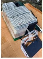
Figure 7: Battery lithium polymer 72 Volts 20 Ah.
