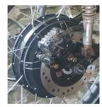
Figure 6: Brush less direct current motor 2,000 watt.
