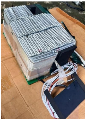
Figure 7: Battery lithium polymer 72 Volts 20 Ah.
