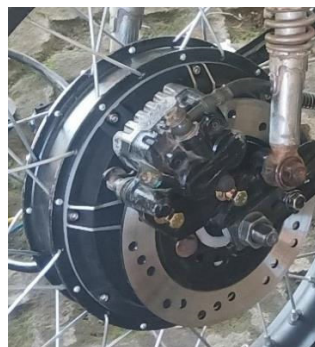
Figure 6: Brush less direct current motor 2,000 watt.
