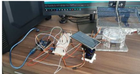
Fig. 2. Developed the prototype of proposed system of solar tracker
