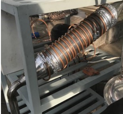
Distilator refrigerasi (evaporator)
