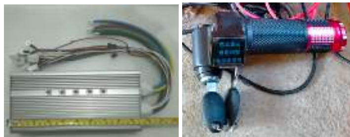
Gambar 5. Controller BLDC 4.800W dan throttle gas
