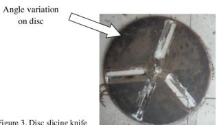
Figure 3. Disc slicing knife
