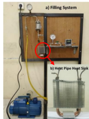
Figure 1. Mechanism of injected fluid into the heat pipe: a) Filling system, b) heat pipe which already injected with methanol working fluid.
