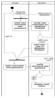
Fig. 2. Activity Diagram Register New User And Sign In
