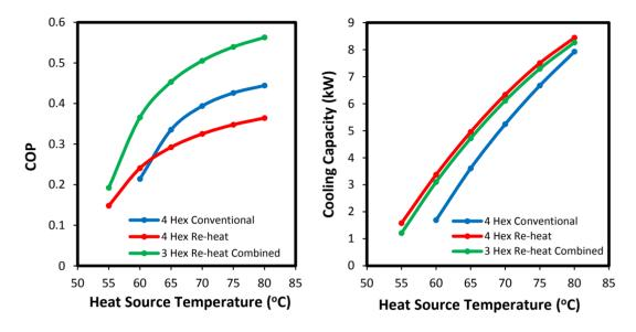
Fig. 3. The COP comparison on the effect of heat source temperature
