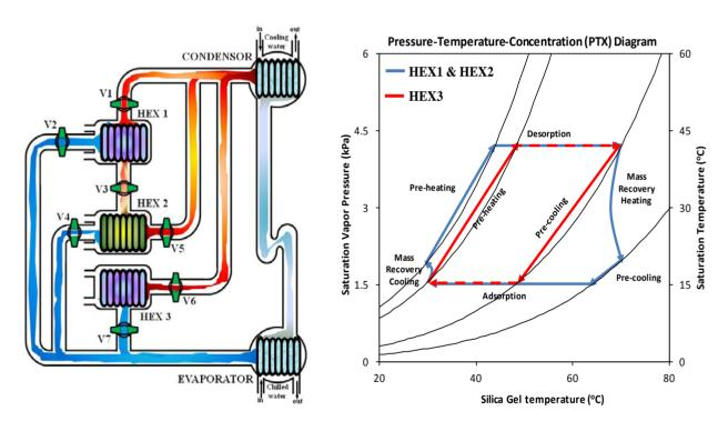
Fig. 1. The cycle schematic of the proposed chiller and the PTX diagram
