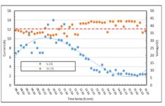
Figure 4: Variation of daily Current (I) and Voltage (V) of the photovoltaic array.
