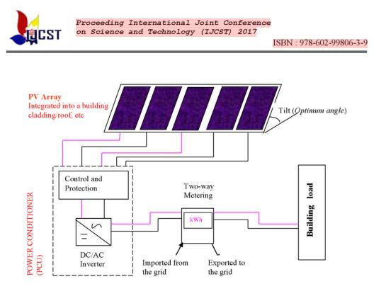
Figure 2. Building Integrated Photovoltaic design
