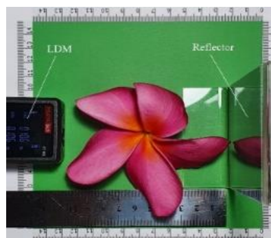
Figure 4. Manual measurement of petal flower dimension using laser distance meter (LDM)
