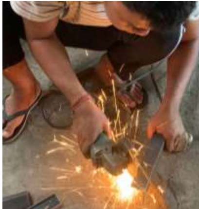
Gambar 4.10 Proses pemotongan rangka cover rantai
