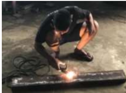
Gambar 4.11 Proses pengelasan cover rantai
