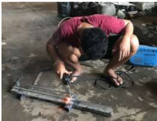
Gambar 4.6 Proses pengelasan besi stainless
