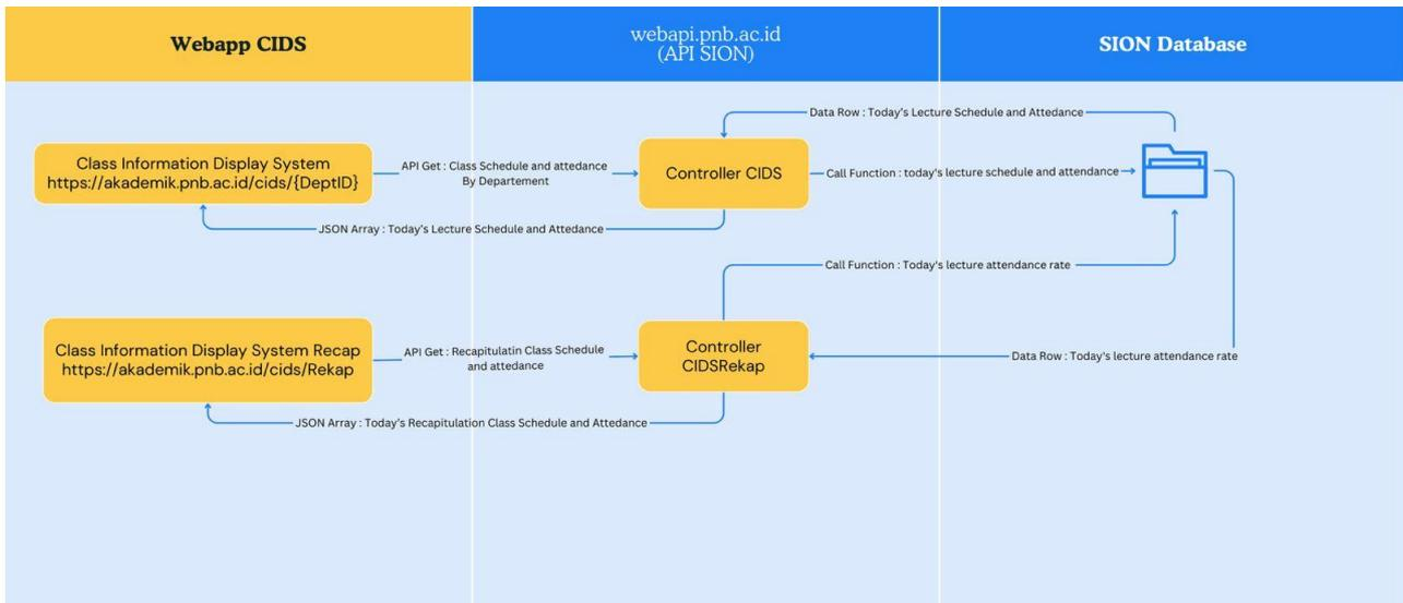
**Figure 2.** Information Display System Class Processing Flow with WebApi
