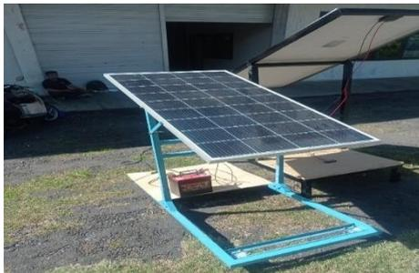
Gambar 18 Rangka panel surya
