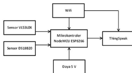
Figure 1. Monitoring System Hardware Block Diagram
