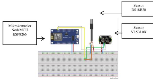
Figure 4. Thingspeak Wiring Diagram with Fritzing
