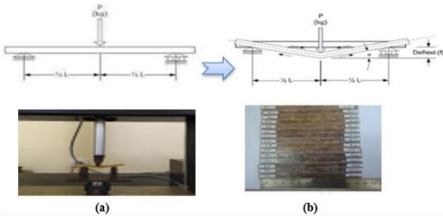
Figure 5. (a) Flexural strength test apparatus and (b) test specimen.
