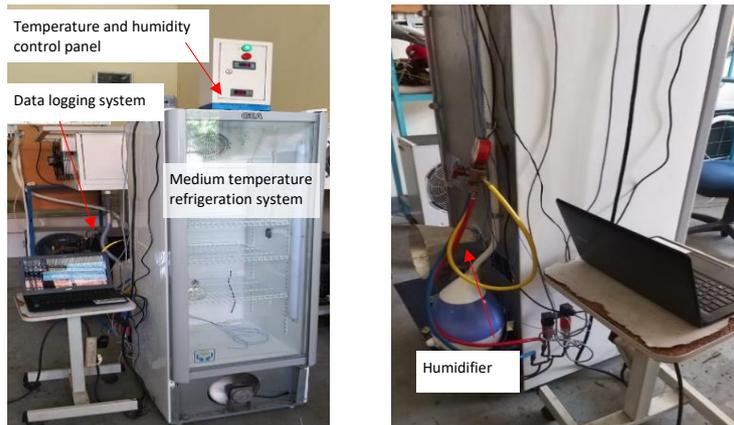
**Fig. 1. Medium temperature refrigerator test rig**
