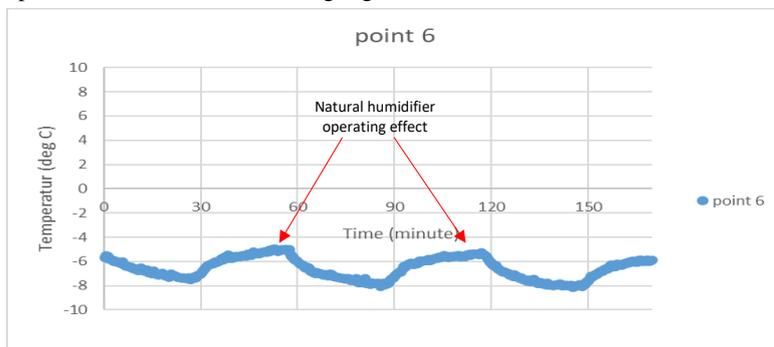
Fig. 7. Temperature increasing on humidifier operating (set 0°C)
