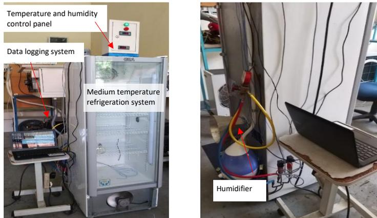
**Fig. 1. Medium temperature refrigerator test rig**
