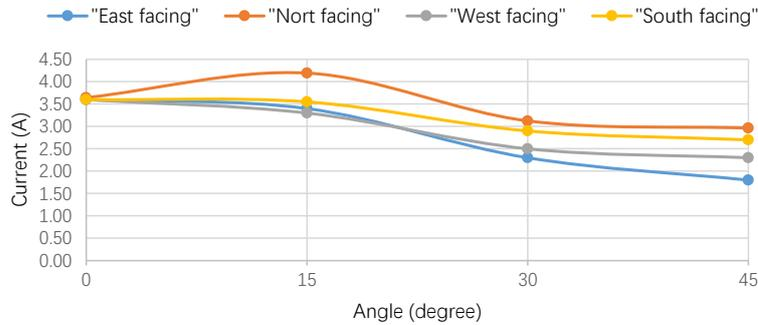
**Fig. 4. Variation of current (I) output with combination of facing and angles of photovoltaic array at Bali State Polytechnic-Bali Indonesia**
