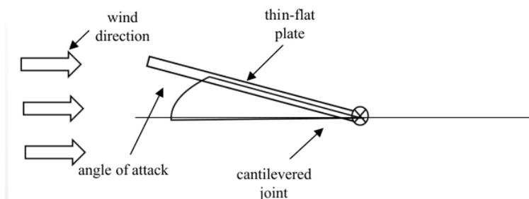
Figure 1. Experimental setup diagram
