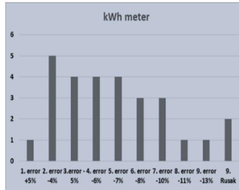
Gambar 5. Diagram persentase error kWh meter
