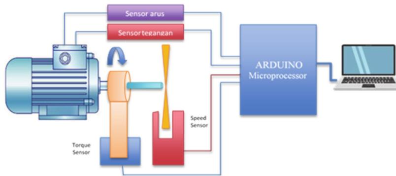
Figure 4: Speed and torque measuring circuit.
