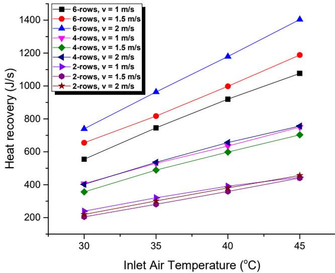
Fig. 5 Heat recovery on evaporator HPHE
