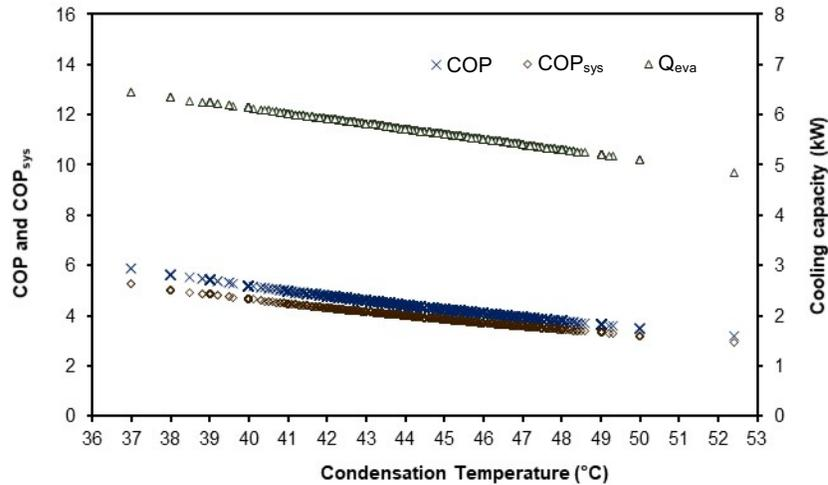
FIGURE 4. Effects of condensation temperature on energy performances (COP,  $COP_{sys}$  and  $Q_{eva}$ ) of the AC system
