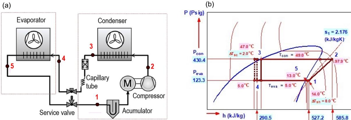
**FIGURE 1.** (a) Simplified schematic of the residential AC system completed with points of investigation; (b) Log pressure and enthalpy diagram of the AC system with R-32 refrigerant, investigated at evaporation temperature ( $T_{eva}$ ) 5 °C and condensation temperature ( $T_{con}$ ) 49 °C
