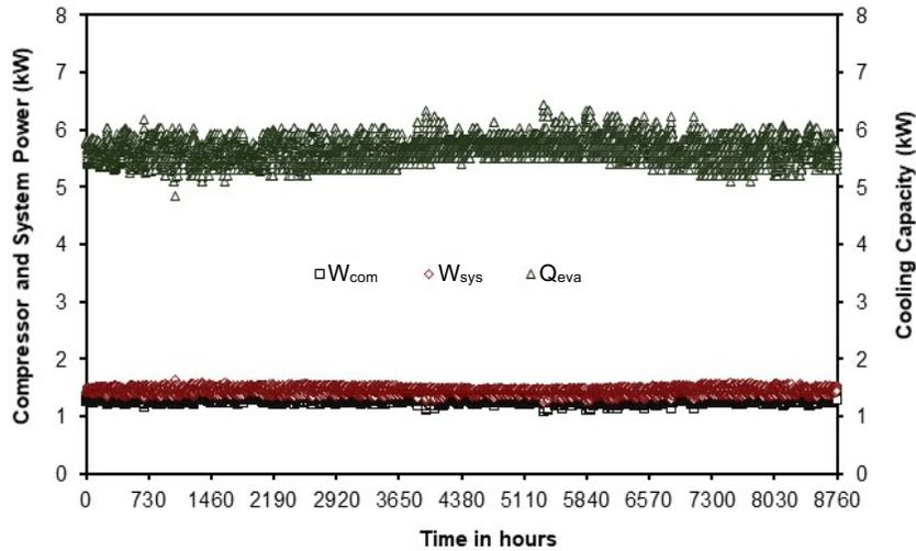
**FIGURE 6.** Seasonal cooling capacity, power consumption of the compressor and overall AC system
