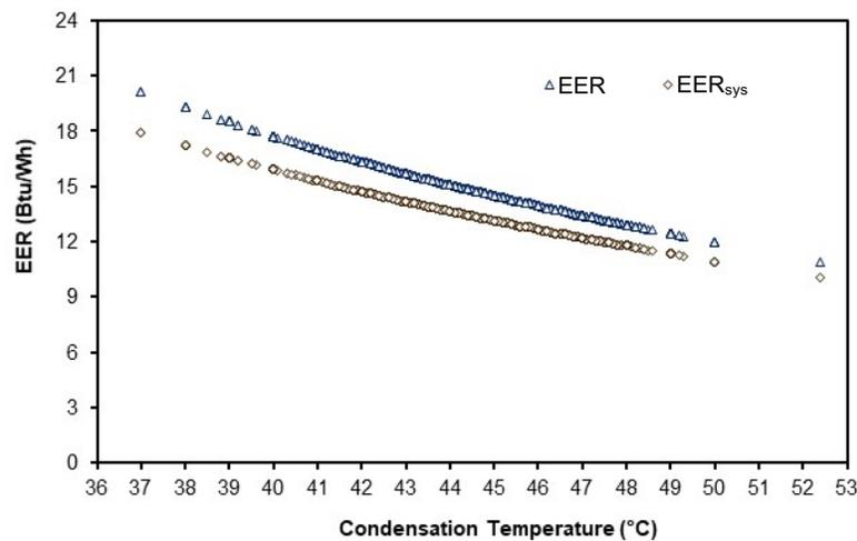
FIGURE 5. Effects of condensation temperature on energy efficiency ratio (EER and  $EER_{sys}$ ) of the AC system
