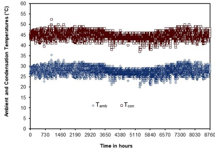
FIGURE 2. Seasonal ambient and condensation temperatures ( $T_{amb}$  and  $T_{con}$ )
