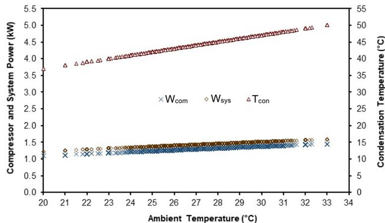
FIGURE 3. Effects of ambient temperature on the compressor power and AC system power consumption
