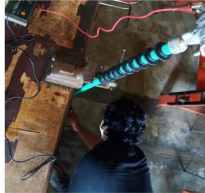
Figure 4: Wet insulation resistance pretest with megger 10,000 volt.
