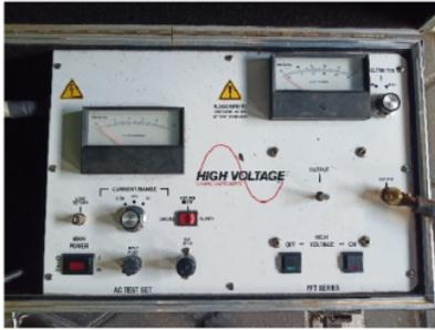
Figure 5: High voltage VLF hi-pot instruments.
