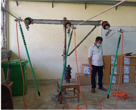
Figure 2: Electrical safety grounding on the trial.
