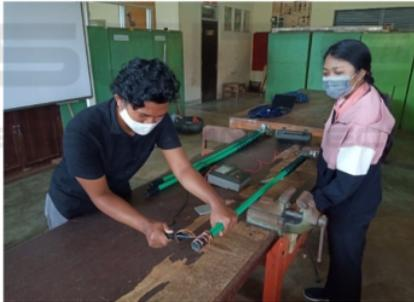
Figure 3: Dry insulation resistance pretest with megger 10,000 volt.
