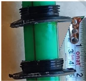
Figure 8: Rubber Ring on The Safety Grounding Shaft.
