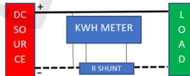
Figure 4: Installation circuit DC digital KWH meter.
