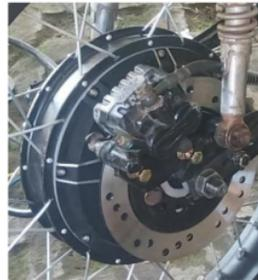
Figure 6: Brush less direct current motor 2,000 watt.
