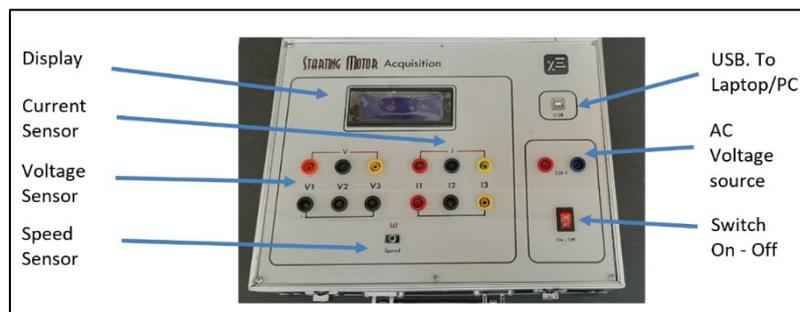
Figure 8. Front panel of starting motor acquisition module.
