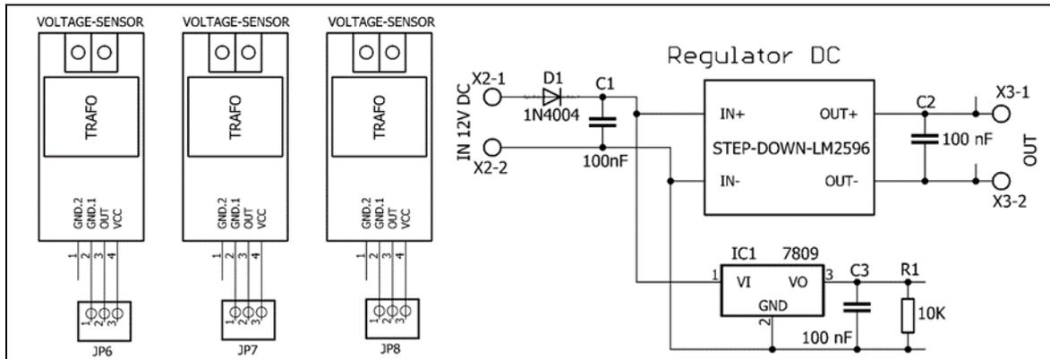
Figure 3. Voltage sensor and DC Regulator circuit diagram.
