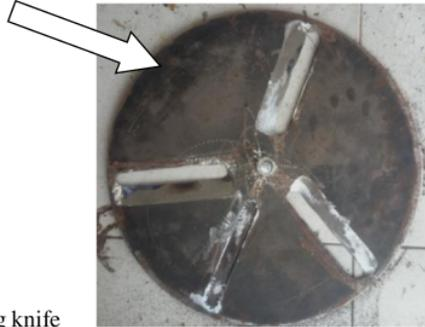
Figure 3. Disc slicing knife
