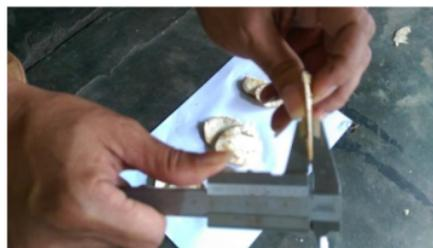
Figure 5. Measuring the thickness of the slices
