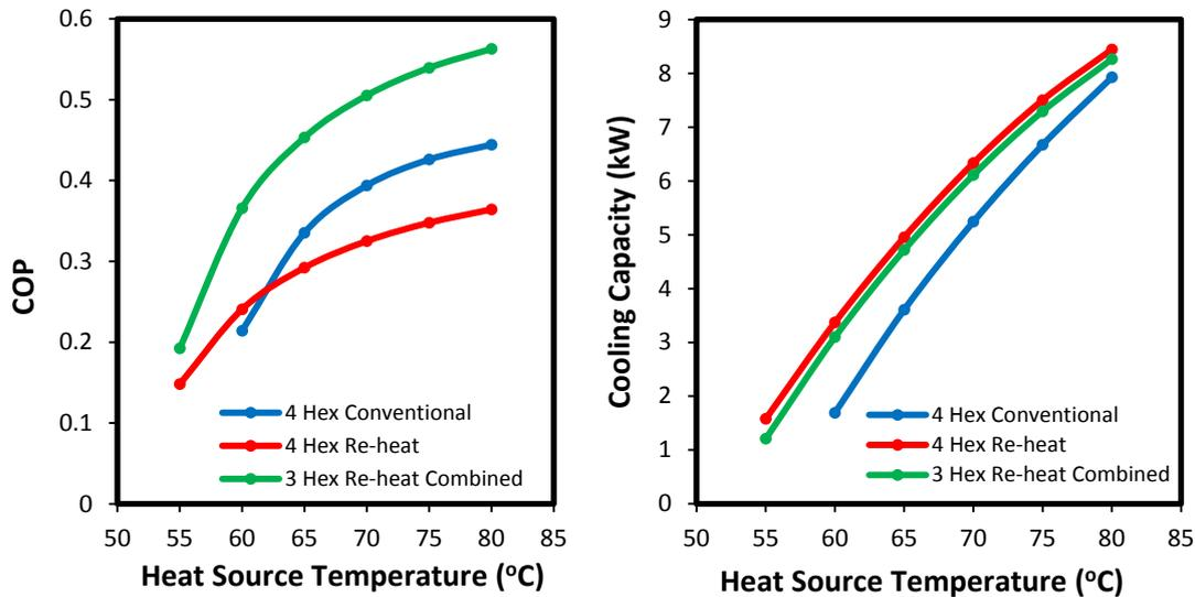
Fig. 3. The COP comparison on the effect of heat source temperature
