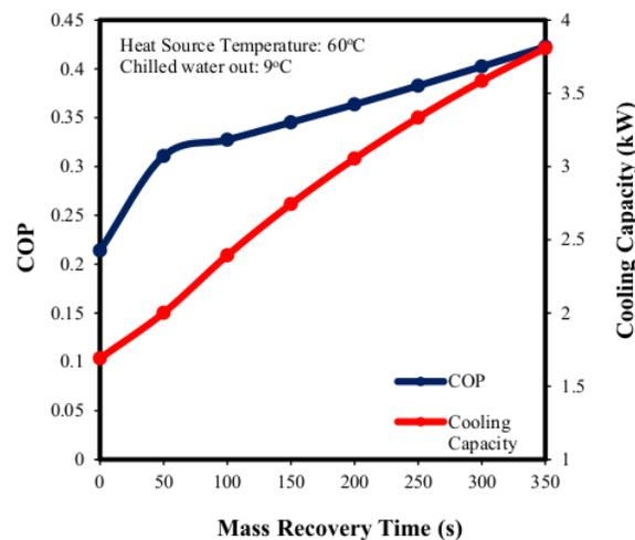
Fig. 2. The effect of Mass Recovery Time on COP and cooling capacity
