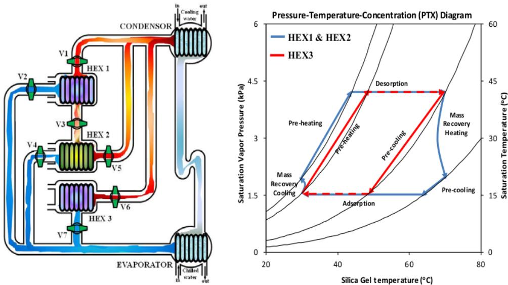
Fig. 1. The cycle schematic of the proposed chiller and the PTX diagram
