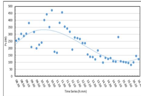
Figure 5: Variation of daily power output of photovoltaic.
